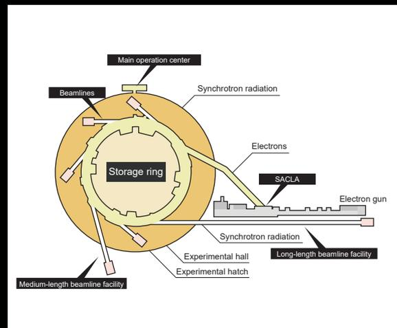
Internal structure of SPring-8
