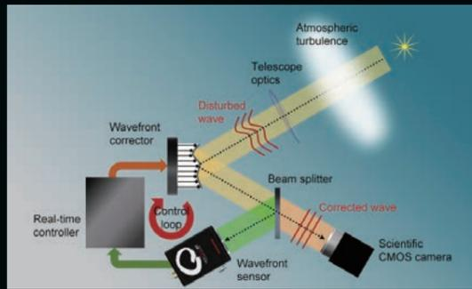
As the phase can be measured directly, errors are less likely to occur. Since adaptive optics for direct imaging of exoplanets requires high-speed and high-precision wavefront control, so does wavefront measurement. Improving the performance of wavefront sensors is essential for the evolution of adaptive optics.
